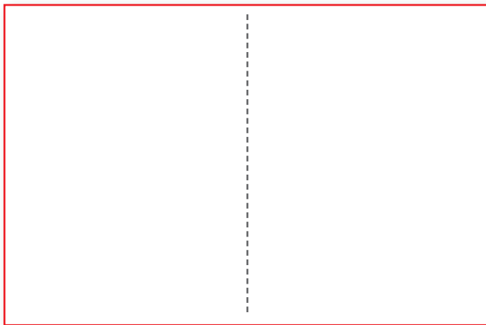
Double Page Spread (DPS) 420mm x 297mm (+ 3mm bleed = 426mm x 303mm)
